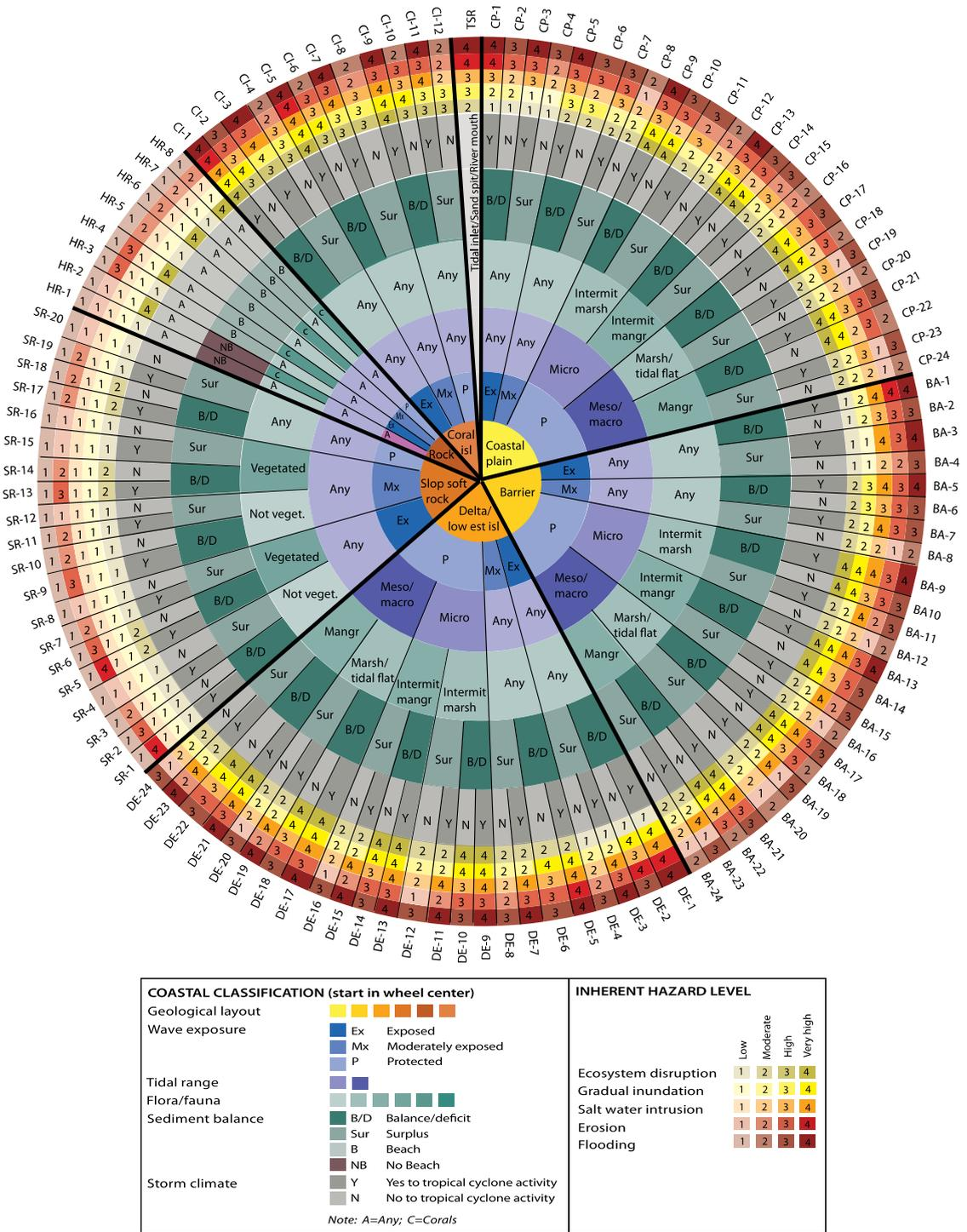
**Fig. 1.** The Coastal Hazard Wheel consisting of six geo-biophysical classification circles, five hazard circles and the coastal classification codes. In the classification code, CP stands for coastal plain, BA for barrier, DE for delta, SR for sloping soft rock, HR for sloping hard rock, CI for coral island and TSR for tidal inlet/sand spit/river mouth (Rosendahl Appelquist, 2012).
