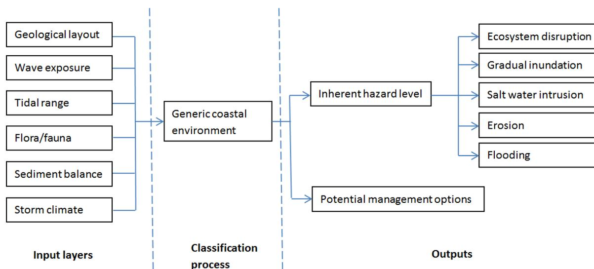
**Figure 3:** Schematic illustration of the functioning of the Coastal Hazard Wheel methodology
