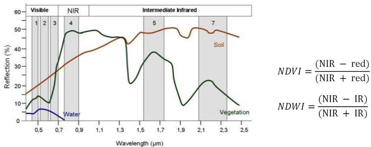
**Figure 14:** Spectral signatures for Soil, water and vegetation (Seos, 2015), the 7 bandwidths measured by Landsat 7, and the formulas for the Normalized Difference Vegetation Index (NDVI) and Normalized Difference Water Index (NDWI)
