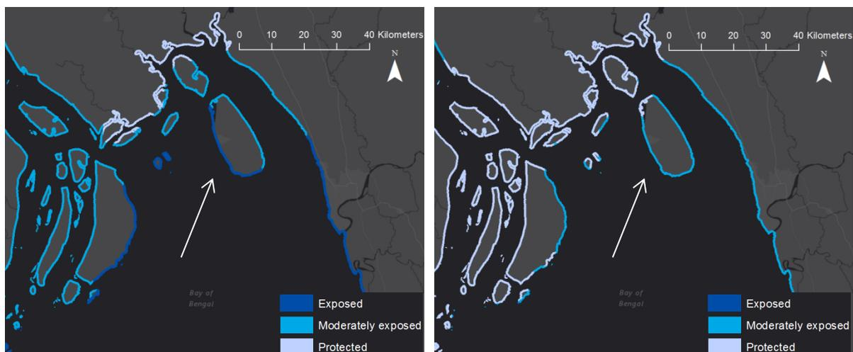
**Figure 18:** The manual (left) and automated (right) free fetch estimation. The white arrows indicates a possible wave direction
