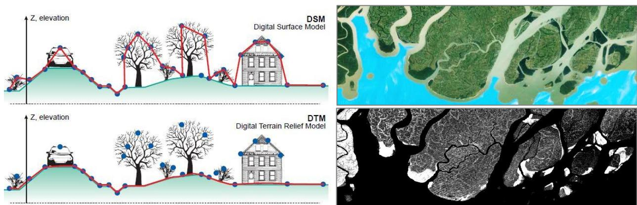
**Figure 13:** Left: The difference between a surface- and an elevation/terrain model (ACP-EU). Upper right: Satellite imagery of a typical coastal environment, showing patches of mangroves and agricultural areas. Lower right: SRTM derived elevation map of the same area in greyscale: black resembles MSL, lighter colors indicate relative height
