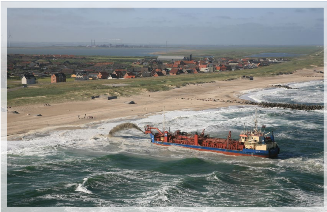
Fig. 1.2. Beach nourishment with Trailing Suction Hopper Dredger and Rainbowing method for transferring nourishment material ashore. Slurry is discharged via a jet at the bow of the ship once it has been sailed as close to the shore as possible (Photo: Rohde Nielsen).
